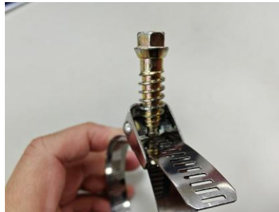
Step 2: Pass out the metal tube bundle from under the locking screw
