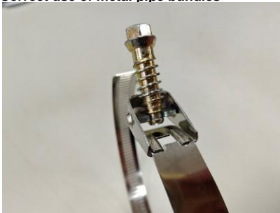
Step 1: Pull up the locking screw as shown in the picture
